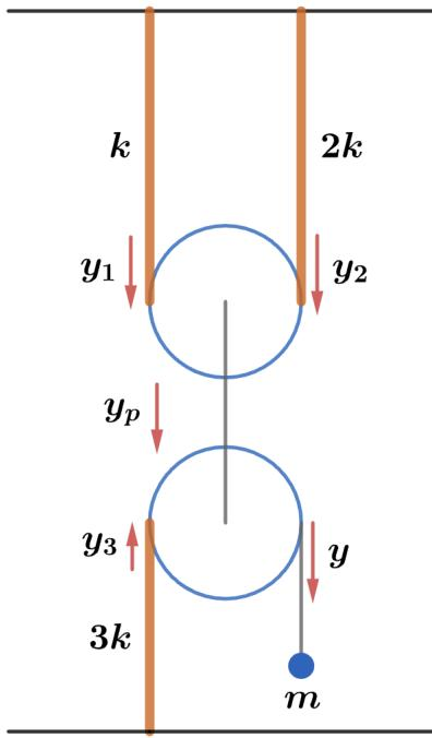
If the pulleys move down by  $y_p$  (they move together to keep the middle string's length fixed) then the total length of the top two springs increases by  $2y_p$ . This has to be equal to their actual increase in length of  $y_1 + y_2$ ,
