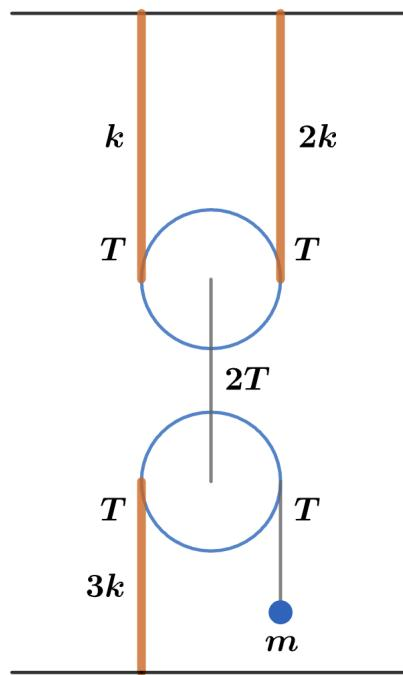
Let  $T$  be the tension in the bottom string (attached to the mass  $m$ ). Then balancing forces on the pulleys, we find the tensions in the springs are also  $T$ . Looking at the mass, we have
