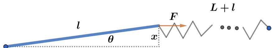
When the spring is moved to the right of the rod, we have a constant spring force  $F = -kl$  pointing to the right (using our given assumption  $L \gg l$ ). If we displace the rod by a small angle  $\theta$ , the restoring torque  $\tau$  is
