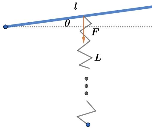
If the spring is moved to the midpoint of the rod, then the moment arm  $l$  is halved to  $l' = l/2$  for the force and torque calculation. The moment of inertia  $I$  is unchanged since the rod is still rotating around the same point. Because we found  $f \propto l$ , we have
