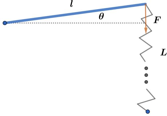
If we displace the rod by a small angle  $\theta$ , then the spring gets stretched by  $x = l\theta$ . The spring force  $F$  is
