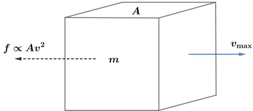
To travel at velocity  $v$  in the presence of air friction  $f$ , we need power
