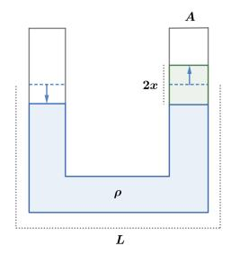
Suppose we displace the water so that the right side moves up by distance x and the left side moves down by distance x. Then the extra weight on the right side is
