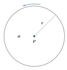
Let  $\lambda$  be the maximum kinetic energy per kilogram that can be stored in the flywheel. If we double the thickness h of the flywheel, that is equivalent to stacking two flywheels on top of each other. Since each has  $\lambda$  energy per kilogram, the combination also has  $\lambda$  energy per kilogram. Hence,  $\lambda$  is independent of h.
