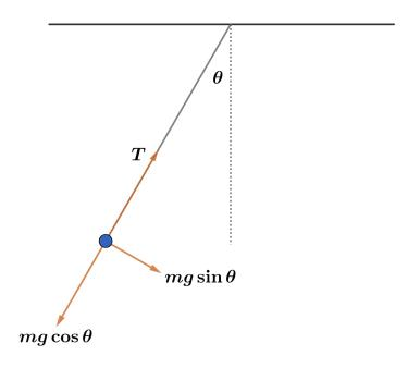
The pendulum feels the forces of tension and gravity. Applying Newton's 2nd law in the tangential direction,
