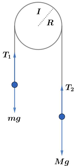
We first find the acceleration in an Atwood machine where the pulley has moment of inertia  $I$ . Applying Newton's 2nd law to each mass and the pulley,
