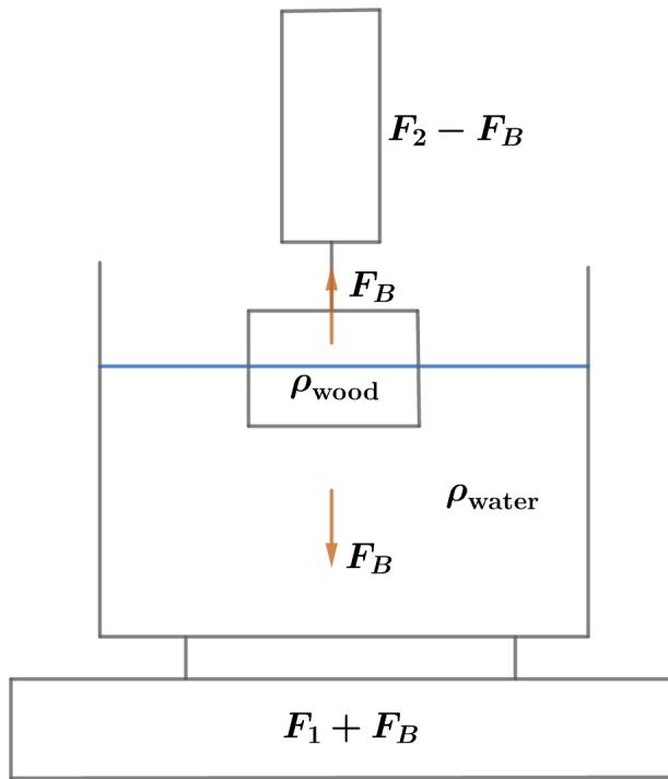
Once the block is submerged in the water, the buoyant force  $F_B$  acts upward on the block reducing the tension to  $T = F_2 - F_B$ . By Newton's 3rd law, the block also exerts a force  $F_B$  down on the water so the normal force on the bottom increases to  $N = F_1 + F_B$ .
