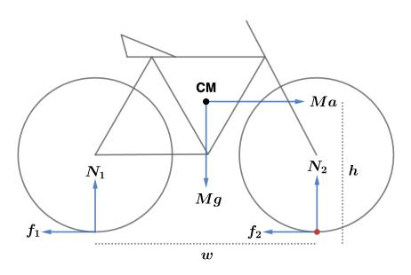
We go to the accelerating frame to reduce the setup to a statics problem, introducing the fictitious inertial force  $-M\vec{a}$  on the bicycle's CM. Choosing the contact point of the front wheel with the ground as the pivot point, we can balance torques:
