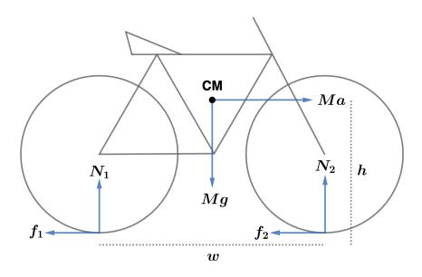
We go to the accelerating frame to reduce the setup to a statics problem, introducing the fictitious inertial force  $-M\vec{a}$  on the bicycle's CM. Choosing the CM as the pivot point, we can balance torques:
