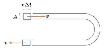
To find the force the stream of water exerts on the U-tube, we consider a small time interval  $\Delta t$ where a small mass  $\Delta m$  of water enters from the left at the top of the U-tube. Since the water is flowing at velocity v, the length of this segment is  $\Delta L = v\Delta t$  so
