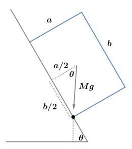
For the block to stay at rest, there should be no torque. This means the weight vector (acting at the center of mass) should pass through the pivot point to have zero moment arm. By using similar triangles in the figure, we find
