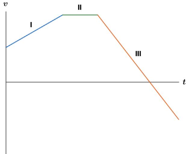
Since the acceleration is given by the slope of a velocity-time graph, we see the car travels at three different accelerations from beginning to end. From the graph, the car has a small positive acceleration for part I of the motion, zero acceleration for part II, and a large negative acceleration for part III. Thus, the answer is C.
