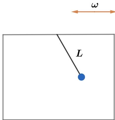
The final amplitude is maximized when the box is shaken at the resonant frequency:
