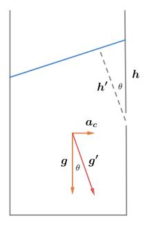
In the noninertial frame of the beaker, we can include the contribution from the centrifugal force into effective gravity g' that points at an angle  $\theta$  from the vertical. We have from similar triangles,
