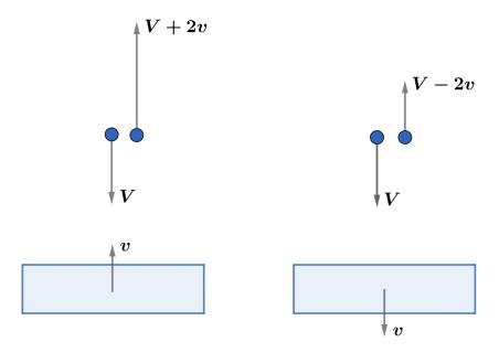
If the ball collides with the plate when it is traveling upward, the ball's speed increases by 2v after the collision, which can be seen by going to the frame of the plate. Similarly, if the ball collides with the plate when it is traveling downward, the ball's speed decreases by 2v after the collision.
