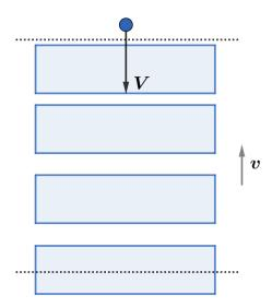
If the plate is moving up at any location, then the ball's speed will increase after it collides with the plate.
