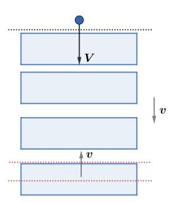
If the plate is moving down, then most of the time the ball's speed will decrease after it collides with the plate. However, if the plate is near the bottom of the region, then it has time to reverse direction as the ball moves through the region. The subsequent collision would then increase the speed of the ball.
