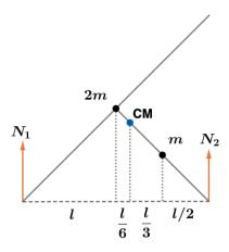
We first find the horizontal location of the CM for this object. We can replace the two rods connected in a line with a point mass 2m at their center. We can replace the third rod with a point mass m located at its center.
