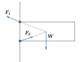
Consider an idealization where the platform is attached to the wall only at the top and bottom points of its side. The vertical component of the forces must point up to balance gravity. For the total torque to be zero, the two forces  $F_1, F_2$  and the weight W vector must intersect through the same point. Thus, there is tension in the top and compression in the bottom so the answer is C.
