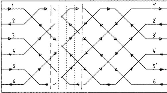
**Figure 3.** A network with  $M = 6, N = 4$  and strip boundary conditions, connected to semi-infinite, ideal conductors. Arrows indicate direction of current flow. A ‘slice’ of the system is contained between broken lines; sub-slices corresponding to the matrices **A**, **B**, **C** and **D** (equation (9)) are contained between dotted lines. The transfer matrix relates amplitudes on the links marked 1, 2, . . . , 6 to those on the links marked 1', 2', . . . , 6'.
