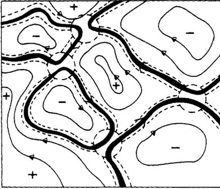
**Figure 1.** Sketch of a typical potential,  $V(x, y)$ . Full curves represent equipotentials and arrows give direction of guiding centre motion; + and - denote maxima and minima. Heavy curves indicate contours at potential  $V_0$ . Portions of these contours are enclosed in strips and circles (broken lines) which correspond to links and nodes of the network model.
