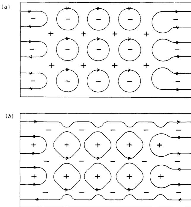
**Figure 4.** The network of figure 3 reduces to a set of disconnected loops in the tails of the Landau band where quantum tunnelling is negligible and the classical picture is accurate. (a) In the low-energy tail, the loops enclose minima in the potential (-); (b) in the high-energy tail they enclose maxima (+).
