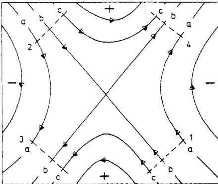
**Figure 2.** Sketch of a saddle point in the potential,  $V(x, y)$ . Full curves represent contours and arrows give direction of guiding centre motion. Amplitudes  $Z_1, Z_2, Z_3$  and  $Z_4$  (see text) are defined on the numbered broken lines. Sets of contours labelled (a), (b) and (c) correspond to potentials  $V_0$  which are, respectively,  $V_0 \ll V_{00}, V_0 \approx V_{00}$  and  $V_0 \gg V_{00}$ , where  $V_{00}$  is the saddle-point potential.
